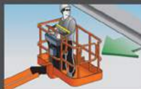
The auto reverse feature activates for most functions
