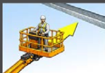
Operator moves towards obstruction.
